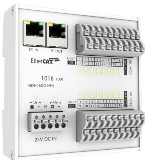
16 x DI, NPN, filter: 3ms 16 x DO, NPN, I max : 0.5A, 24VDC
