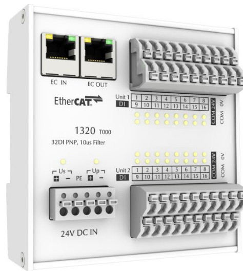
32 x DI, PNP, filter: 10us, 24VDC
