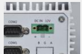
Serial and power interface uses the phoenix terminal tightening
