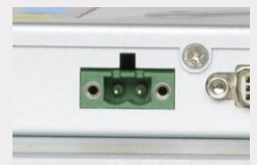
Phoenix terminal using fastening type power connector
